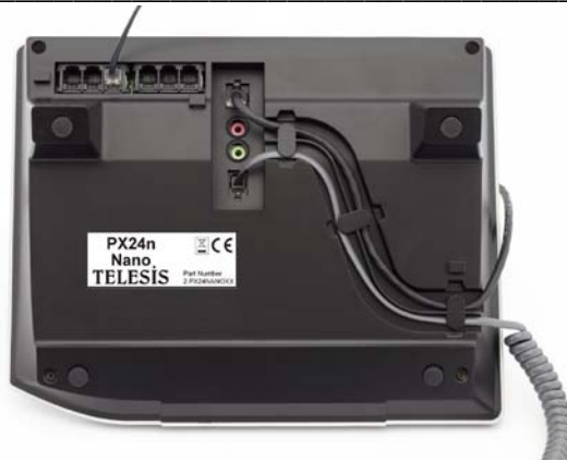
FXS, FXO, power, headset, microphone, handset connectors are located at the bottom.
